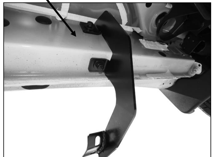
(Fig 4) Driver/left front Bracket installed
