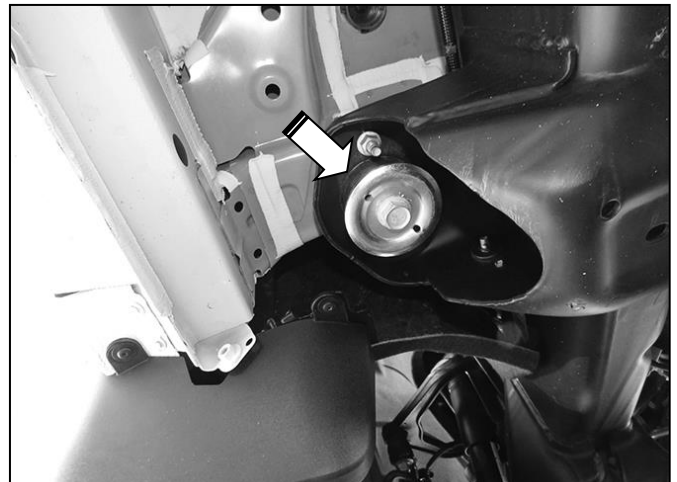
(Fig 2) Driver/Left front mounting location (2020 25-3500 model with cupped body bolt washer shown)
