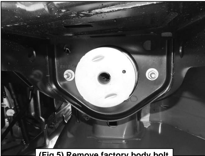
(Fig 5) Remove factory body bolt
